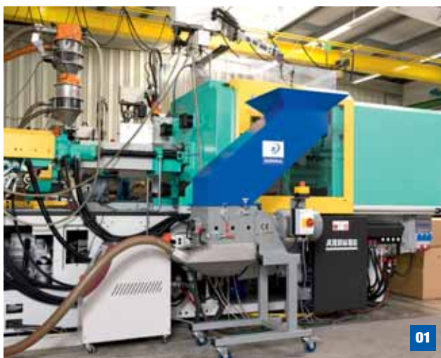
01 GSL slow speed granulator working inline next to the injection machine
